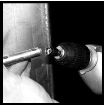
Use a 5/16" Hex Nut Driver in a power drill
